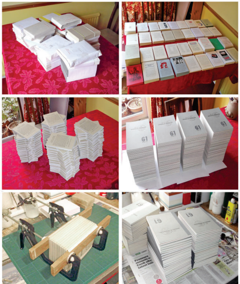
Assembling the 2015 edition took about two weeks: (a) A heap of parcels from around the world. (b) Pages ready for collating. (c) Pages collated and stacked. (d) Covers and prelims added. (e) Binding. (f) Completed books.
